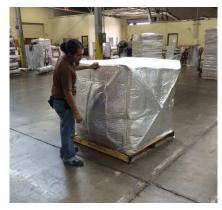
2. We recommend using bungee cord or tape to cinch the bottom edge to prevent airflow entering from below. Alternatively, you can simply tuck the bottom edges between the pallet and your goods.
