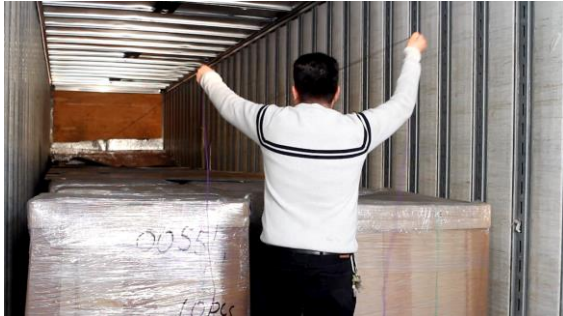
Use ropes to pull the Astro-Quilt all the way out to the final pallets
